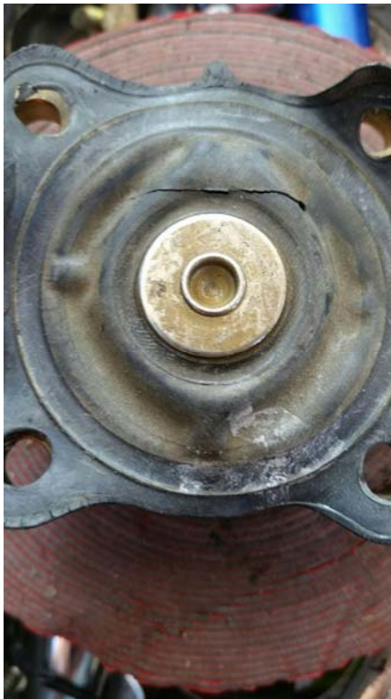
Blown dispenser valve diaphragm
