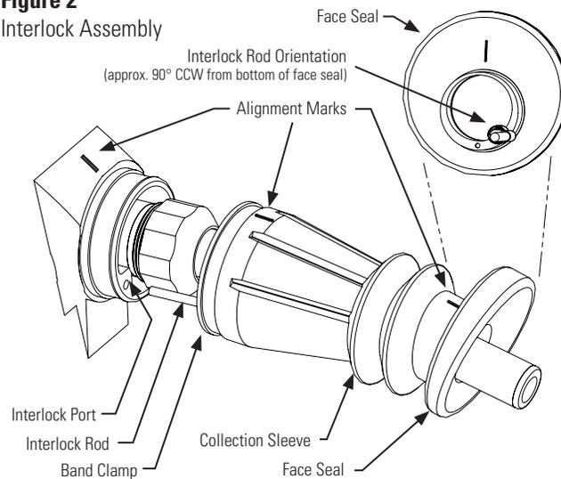
The nozzle will not operate properly if vent hole becomes clogged. The nozzle will not function properly without the interlock rod properly engaged. Keep the hose connections tight.
