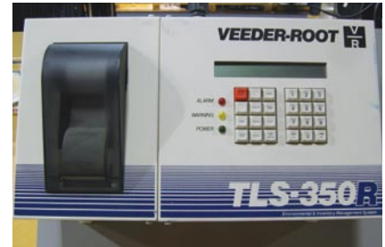
Veeder-Root In-Station Diagnostics
